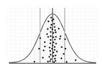
Combining new A-D technology with multi-channel control produces extremely precise internal weight information. Resultant data is sampled and evaluated statistically to determine the sample mean and standard deviation. This vital information is then used to optimize filter averaging and filter cutoff bands to maximize both data stability and response to true weight changes.
